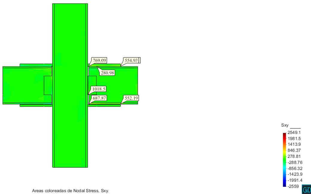
Figure 112: Shear stresses (XY plane, SXY) in M2-A572 conventional model.
