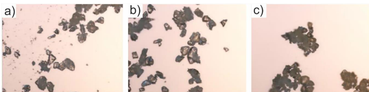
Figure 53. Optical microscope images (x100) of a) IL-gel support before infiltration, b) IL-gel infiltrated with 100 wt% [EMIM][NTf 2 ], and c) IL-gel infiltrated with 200 wt% [EMIM][NTf 2 ].
