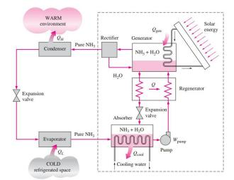
IMAGEN 2: Ammonia absorption refrigeration cycle.
