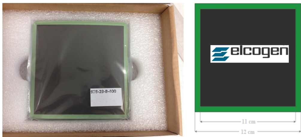
Figure 4.1. Elcogen cells tested in this work, where anode (in green) and cathode (in black) can be distinguished.
