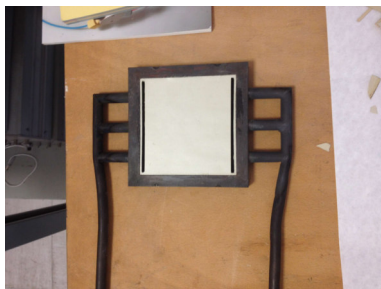
(j) Cathodic internal gaskets (Thermiculite 866LS, 0.4 mm and Thermiculite CL87, 0.35 mm).
