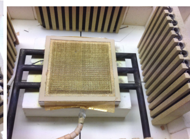
(f) Cell frame (Thermiculite 866LS, 0.4 mm).
