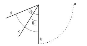
Figure 2. Pendulum diagram used to determine the cutting energy. Source: Author's own elaboration.
