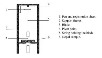
Figure 1. Pendulum for determination of cutting energy. Source: Author's own elaboration.
