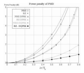
Figure 10. Power Penalty of Polarization Mode Dispersion.
