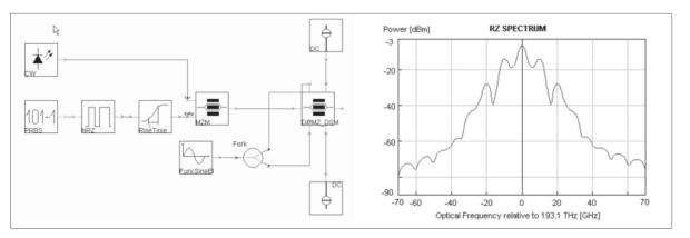
Figure 2. RZ transmitter and its spectrum.
