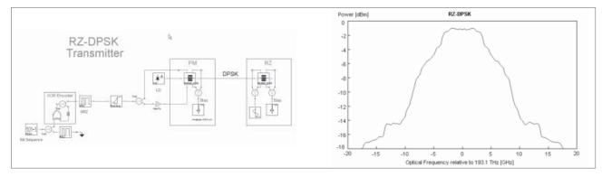
Figure 4. RZ-DPSK transmitter and its spectrum.
