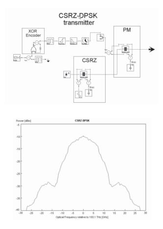
Figure 5. CSRZ-DPSK transmitter and its spectrum.
