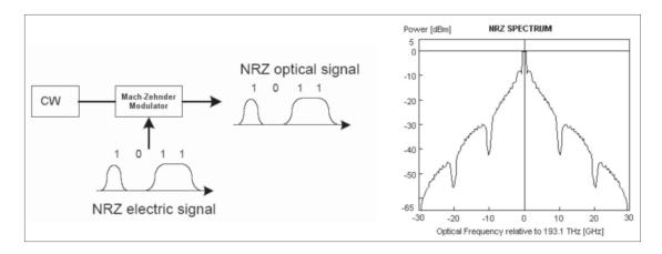
Figure 1. NRZ transmitter diagram and its spectrum.
